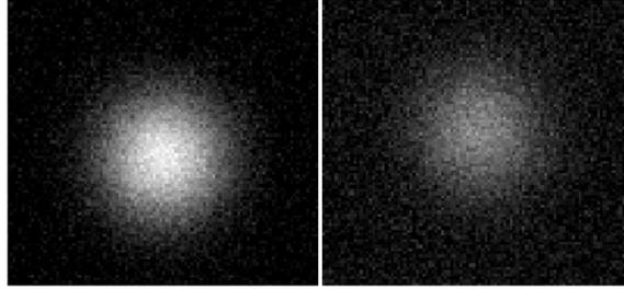
Figure 2 - Simulated star at different SNR's
